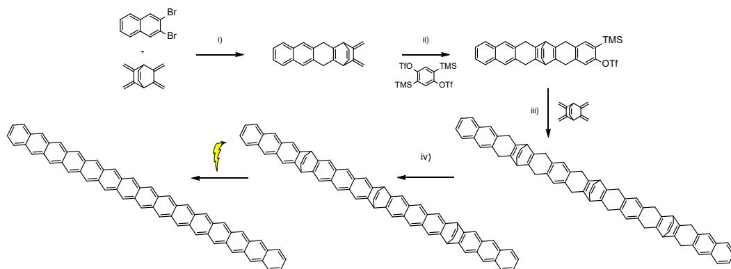
i) n-BuLi, toluene, -60 °C, 3 h; ii) MeCN, CsF, 45 °C, 19 h; iii) DCM, MeCN, KF, 18-crown-6, RT, 16 h; iv) DDQ, CHCl<sub>3</sub>, RT, 2 h; v) Au(111), STM tip, 4 K
